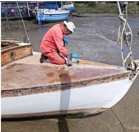
Covering with 2 coats of fibreglass
