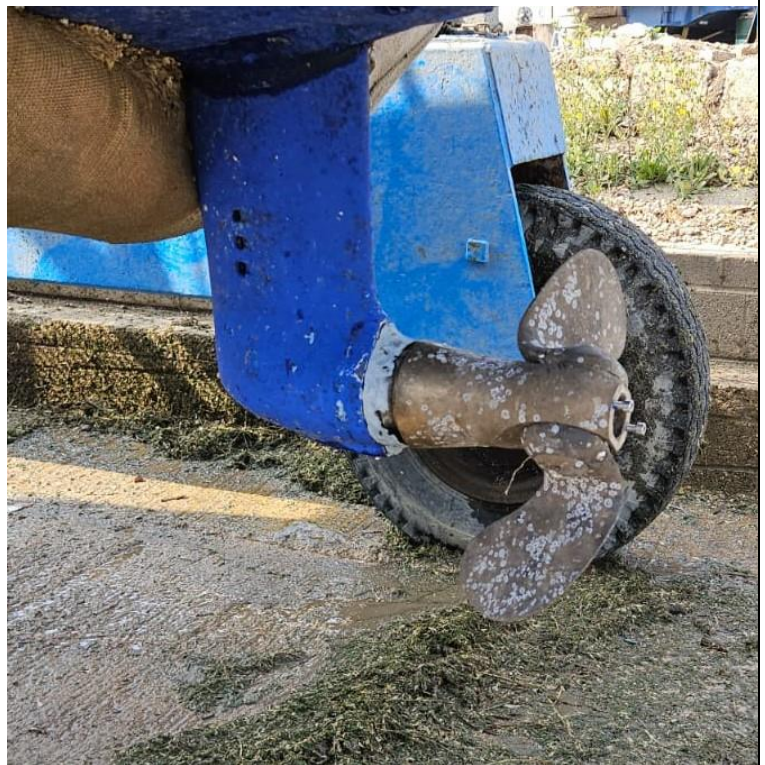
Anode eaten away in 6 months!
